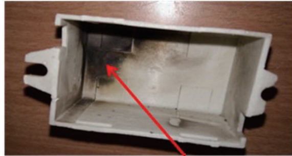
Burnt Mark Under the PCB base cap
