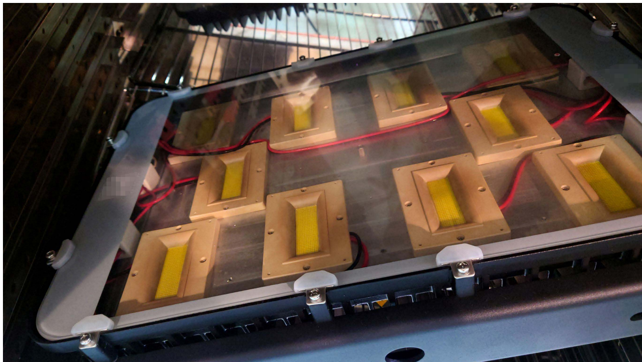
Figure 1. 145°C High-Temperature Functional Validation Test
