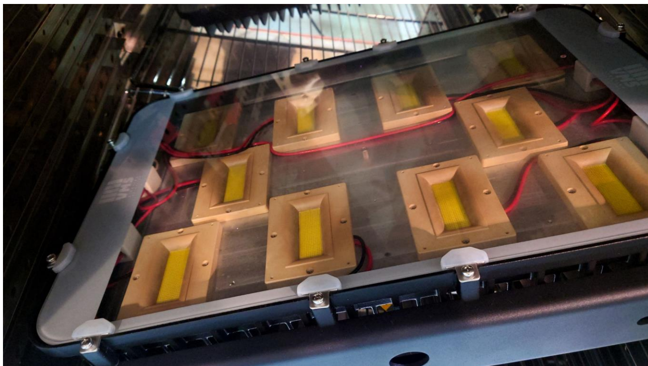
Figure 1. 145°C High-Temperature Functional Validation Test
